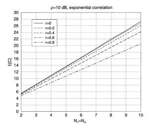
Fig. 4. Mean value of the capacity as a function of  $N_{\rm R}=N_{\rm T}$  for a MIMO system with  $\rho=10$  dB. Exponential correlation case with r ranging from 0 to 0.8
