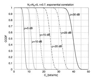
Fig. 2. CCDF of the capacity for a MIMO system with  $N_{\rm T}=5$ ,  $N_{\rm R}=5$ , and  $\rho=5$  to 30 dB. Exponential correlation case with r=0.7.
