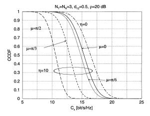
Fig. 5. CCDF of the capacity for a MIMO system with  $N_{\rm T}=N_{\rm R}=4$ , and  $\rho=20$  dB. Correlation model of [15] with  $d_{12}=0.5,\,\eta=0,\,10,$  and  $\mu$  ranging from 0 to  $\pi/2$ .
