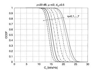
Fig. 6. CCDF of the capacity for a MIMO system with  $N_{\rm T}=N_{\rm R}=4$  ,  $\rho=$ 20 dB,  $\mu=\pi/2$ , and  $d_{12}=0.5$ . Correction model of [15] with  $\eta$  ranging from 0 to 7.
