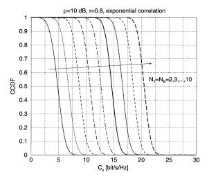
Fig. 3. CCDF of the capacity for a MIMO system with  $\rho=10$  dB. Exponential correlation case with r=0.8, and  $N_{\rm T}=N_{\rm R}=2$  to 10.
