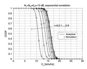
Fig. 1. CCDF of the capacity for a MIMO system with  $N_{\rm T}=6$ ,  $N_{\rm R}=6$ , and SNR per receiving antenna  $\rho=10$  dB. Exponential correlation case with r ranging from 0 to 0.9.
