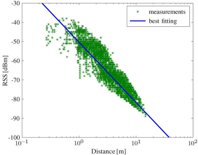
Fig. 3. Measured RSS as a function of the true distance. Best fitting curve is reported with  $P_0 = -50.4$  dBm and  $\beta = 3.14$ .
