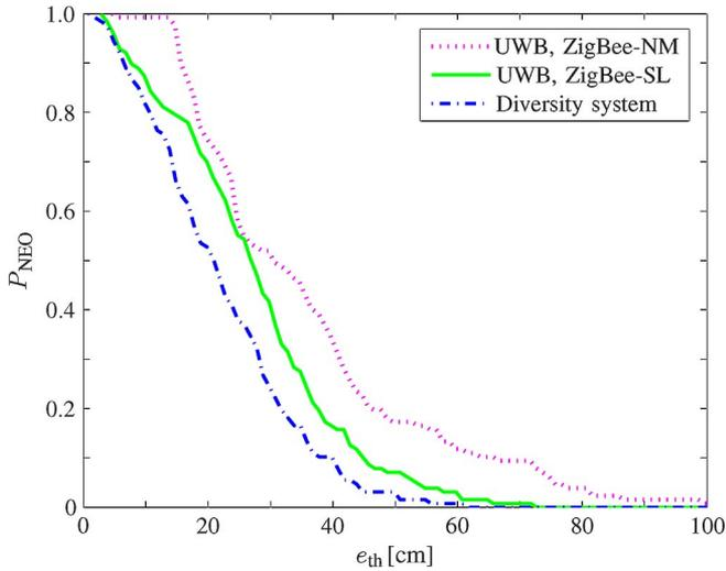
Fig. 11. NEO for UWB and ZigBee technologies with models NM, SL, and SM in variable-speed scenario. Optimum window size is considered for SL.
