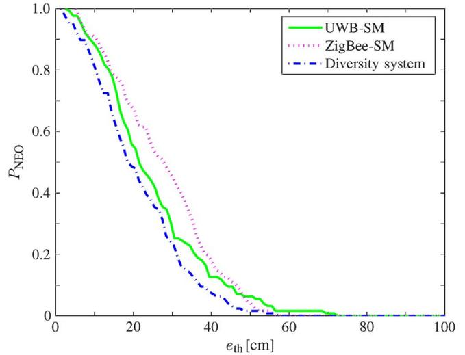
Fig. 10. NEO for UWB, ZigBee, and diversity systems. A variable-speed scenario is considered.
