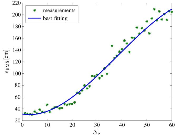
Fig. 5. Navigation RMSE as a function of window size  $N_\nu$  for the UWB system and mobility model SL. A constant-speed scenario is considered.
