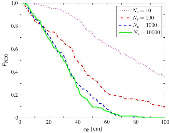
Fig. 4. NEO versus  $e_{th}$  (in centimeters) with  $\Delta_t = 500$  ms for different values of  $N_s$ . The SL model is considered with  $\sigma_m = 0.04$  m and  $N_\nu = 20$ .
