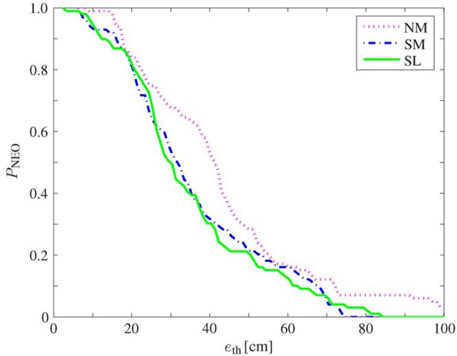
Fig. 7. NEO for the UWB system. Constant-speed scenario. Three mobility models: NM, SM, and SL with optimum window size.
