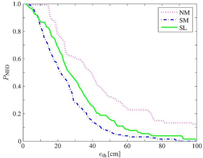
Fig. 8. NEO for the UWB system. Variable-speed scenario. Three mobility models: NM, SM, and SL with optimum window size.
