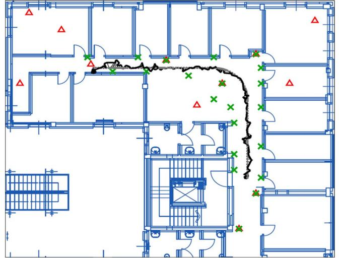
Fig. 12. Real (gray) and estimated (black) trajectories of the robot for the diversity navigation system. UWB (triangles) and ZigBee (crosses) anchors are indicated.
