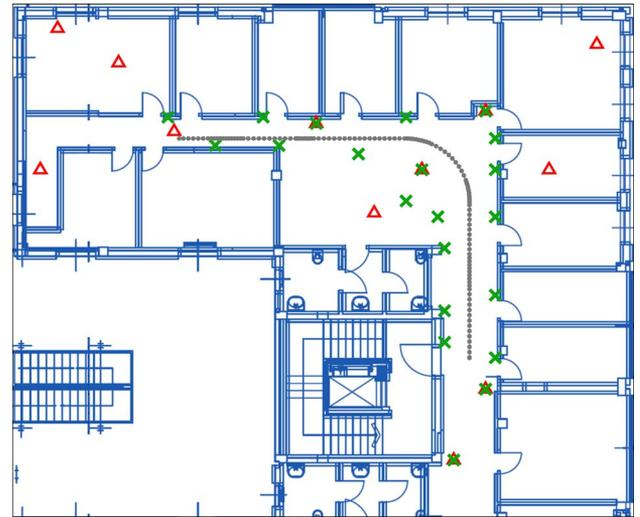
Fig. 1. Experimentation environment with UWB (triangles) and ZigBee (crosses) anchors. The trajectory of the robot is also depicted (gray curve).
