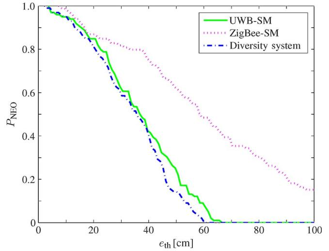
Fig. 9. NEO for UWB, ZigBee, and diversity systems. A constant-speed scenario is considered.
