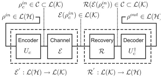
FIG. 1. Transform from standard quantum error correction to quantum spreading channel. By considering the error channel  $\mathcal{E}$  together with the encoding  $U_C$  and the recovery operation  $\mathcal{R}$  with the decoder  $U_C^\dagger$ , the dimension of the SDP may be reduced by a factor of  $(\dim \mathcal{K} / \dim \mathcal{H})^2$ . Note that the output of the encoder  $U_C$  and the recovery channel  $\mathcal{R}$  live on the code subspace  $\mathcal{C}$ .
