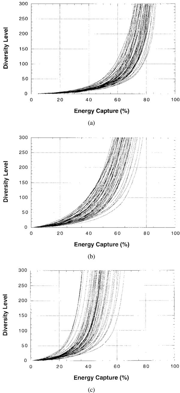
Fig. 2. The required diversity level,  $L_p$ , in a UWB Rake receiver as a function of percentage energy capture for each of the 49 received waveforms in an office representing: (a) a “high SNR” environment; (b) a “low SNR” environment; and (c) an “extremely low SNR” environment.
