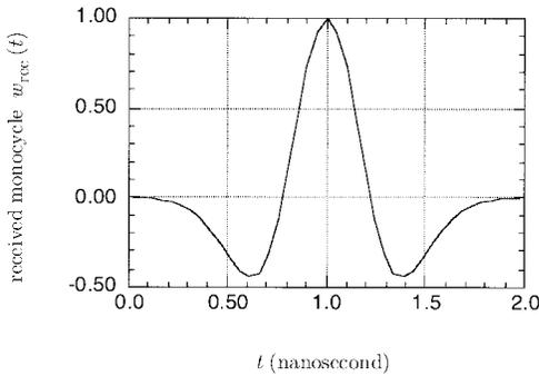
Fig. 1. A typical idealized waveform as a function of time in nanoseconds. The model used in this plot is  $w_{\text{rec}}(t + 1.0) = [1 - 4\pi(t/\tau_m)^2] \exp[-2\pi(t/\tau_m)^2]$  with  $\tau_m = 0.78125$ , which is assumed to be reasonably matched to the isolated paths in the whole ensemble of measured received waveforms.
